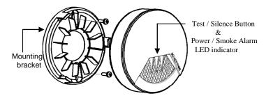
**WARNING:** Do not connect smoke detectors to any other alarm or auxiliary device. Connecting anything else to this detector will keep it from working properly.
